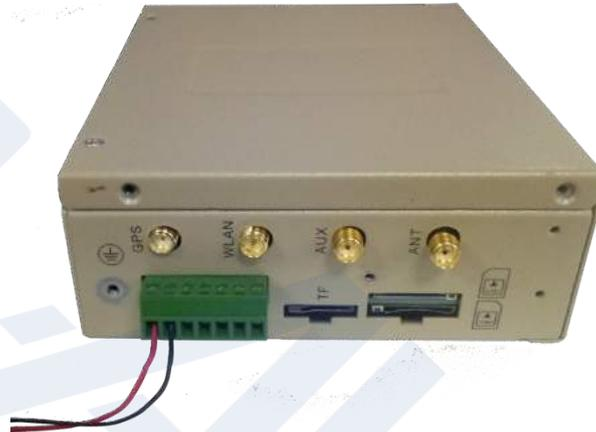
Figure 3-7 Installing the Power Supply
