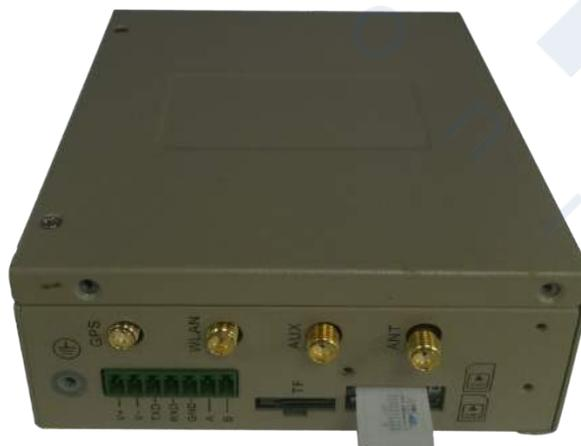
Figure 3-5 Install SIM card
