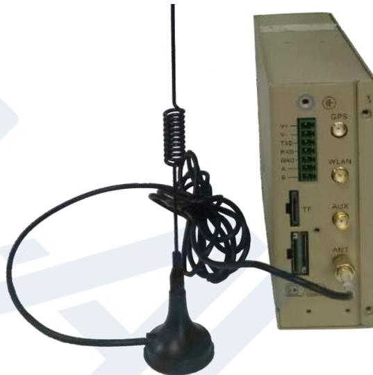
Figure 3-6 Installing an Antenna
