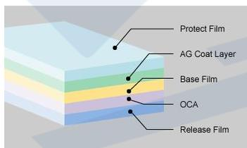
Anti-Vandal film works by protecting the glass substrate from damage and can be easily removed and replaced by new film. This provides a quick on cost-effective solution for those required to maintain public and private spaces from the damage and visual distortion caused by graffiti and reckless vandalism.
