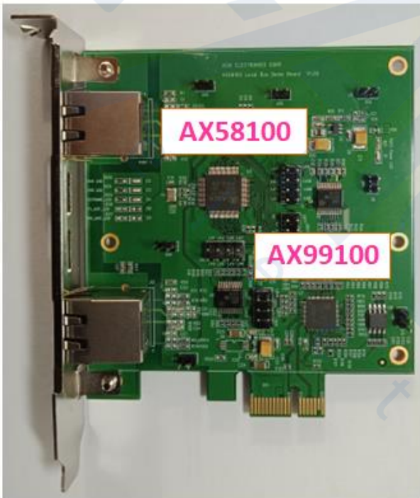
Figure 10. AX58100 + AX99100 Local Bus Demo Kit & Windows SSC/TwinCAT PLC Demo
