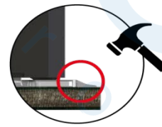
solder meniscus guarantees a robust surfa- ce mount connection
