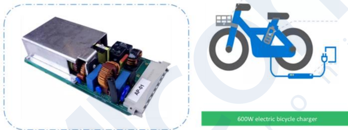
Figure 3: 600W Electric Bike Charging Solution using the HR1211
