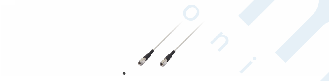
High Performance mmWave Cable Assembly (Rated to 26.5GHz) with 915mm (36'') RG-405 and 2 x 2.92(M) Connectors
