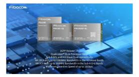
In addition to the Fx190 series, Fibocom launches the FG180(W)/FM180(W)series based on the Snapdragon X72, which supports up to 400MHz bandwidth of NR4CA under mmwave bands, and 200MHz bandwidth of NR 3CA under Sub-6GHz, themaximum downlink rate under the aggregation of the two can reach 4.4Gbps. TheFx180 series is optimized for the FWA market and supports multi-gigabit uplinkand downlink rates.
