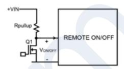
Logic type active mode: DC/DC ON : Q1 OFF
