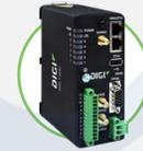
**Digi IX30** is a flexible router designed for critical infrastructure applications. It connects RTUs, PLCs and HMI devices in harsh, remote environments and is optimized for DIN rail or shelf mounting.
