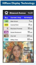
Unlike traditional LCDs that rely on backlighting and can cause eye strain, 0 HiRaso Display Technology reflects ambient light to present clear and paper-like visuals, offering an eye-friendly experience. HiRaso excels in outdoor environments by providing exceptional image quality, ensuring clarity and comfort, where conventional LCDs frequently encounter image distortion and visibility challenges under bright sunlight.
