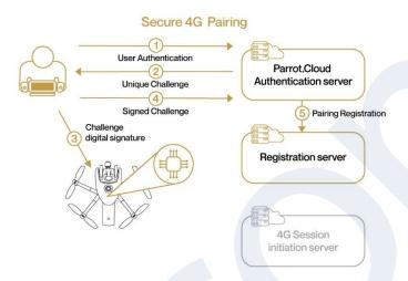
Then, Parrot servers register the association between the user and the drone. When Wi-Fi connection between the user and the drone is lost, ANAFI Ai automatically connects in 4G. ANAFI Ai does a strong authentication on Parrot servers, using its private key stored on the Secure Element. Parrot servers look for the associated users and enables pairing between ANAFI Ai and the Skycontroller 4.
