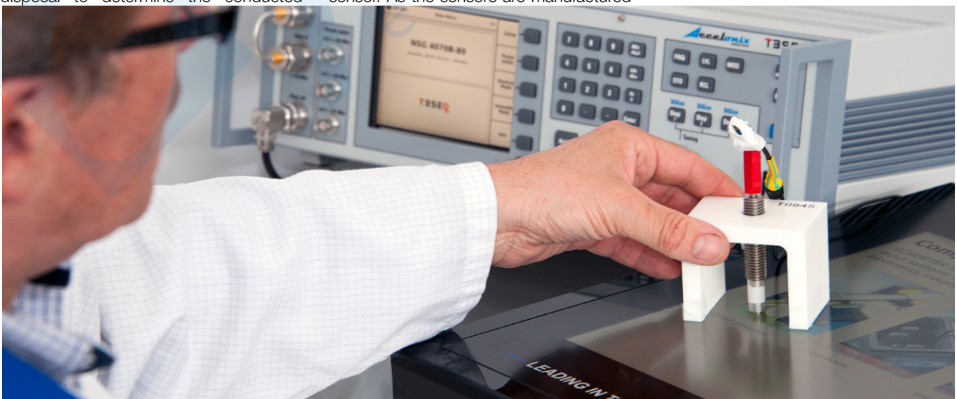
Performing a conducted immunity EMC test
