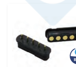
Pogo Pin, Waterproof 5Pin, Pitch 2.5mm T/H 3.0mm, DIP w/o Cap 303C-C3018-25-05
