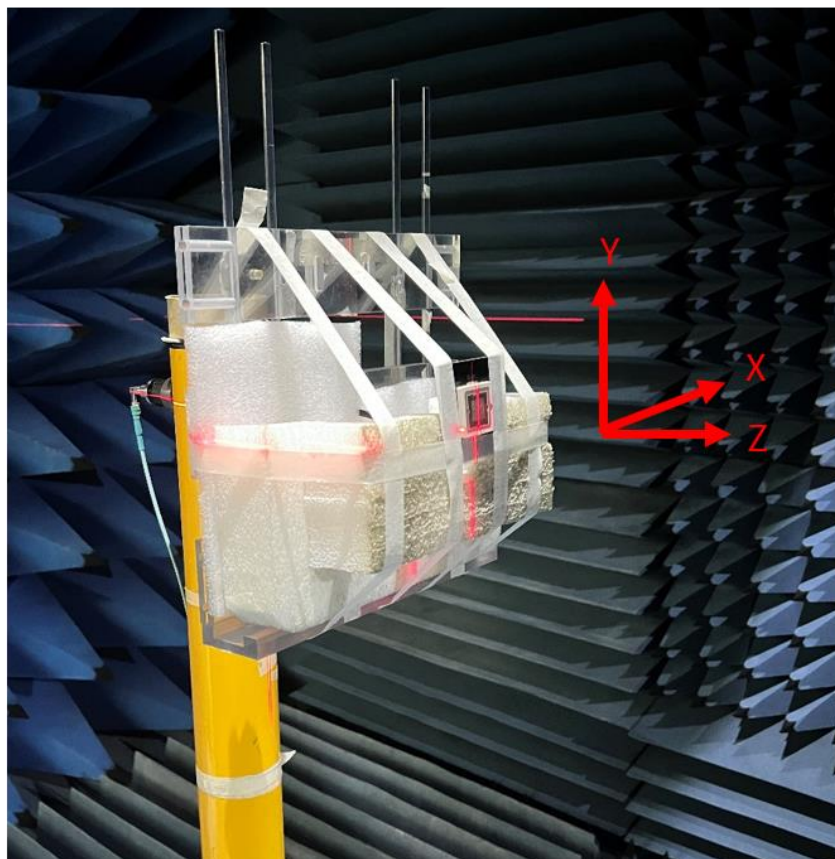
Chamber test setup on 70x70mm ground plane
