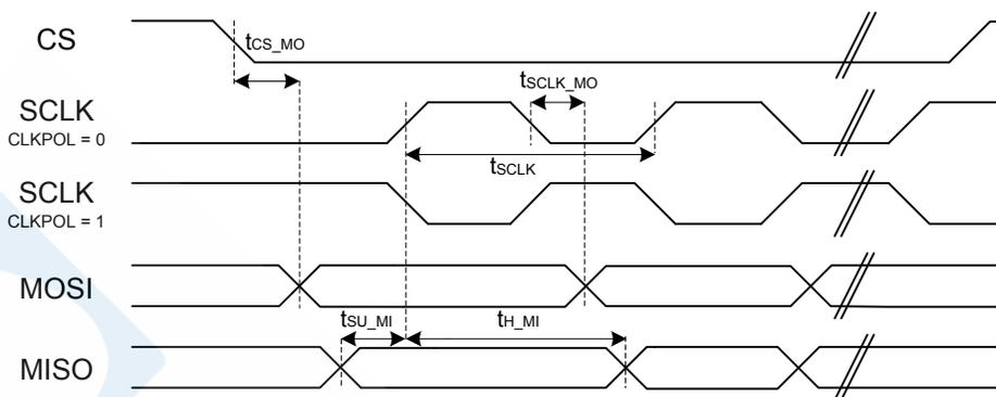
Figure 4.4. SPI Main Timing (SMSDELAY = 0)
