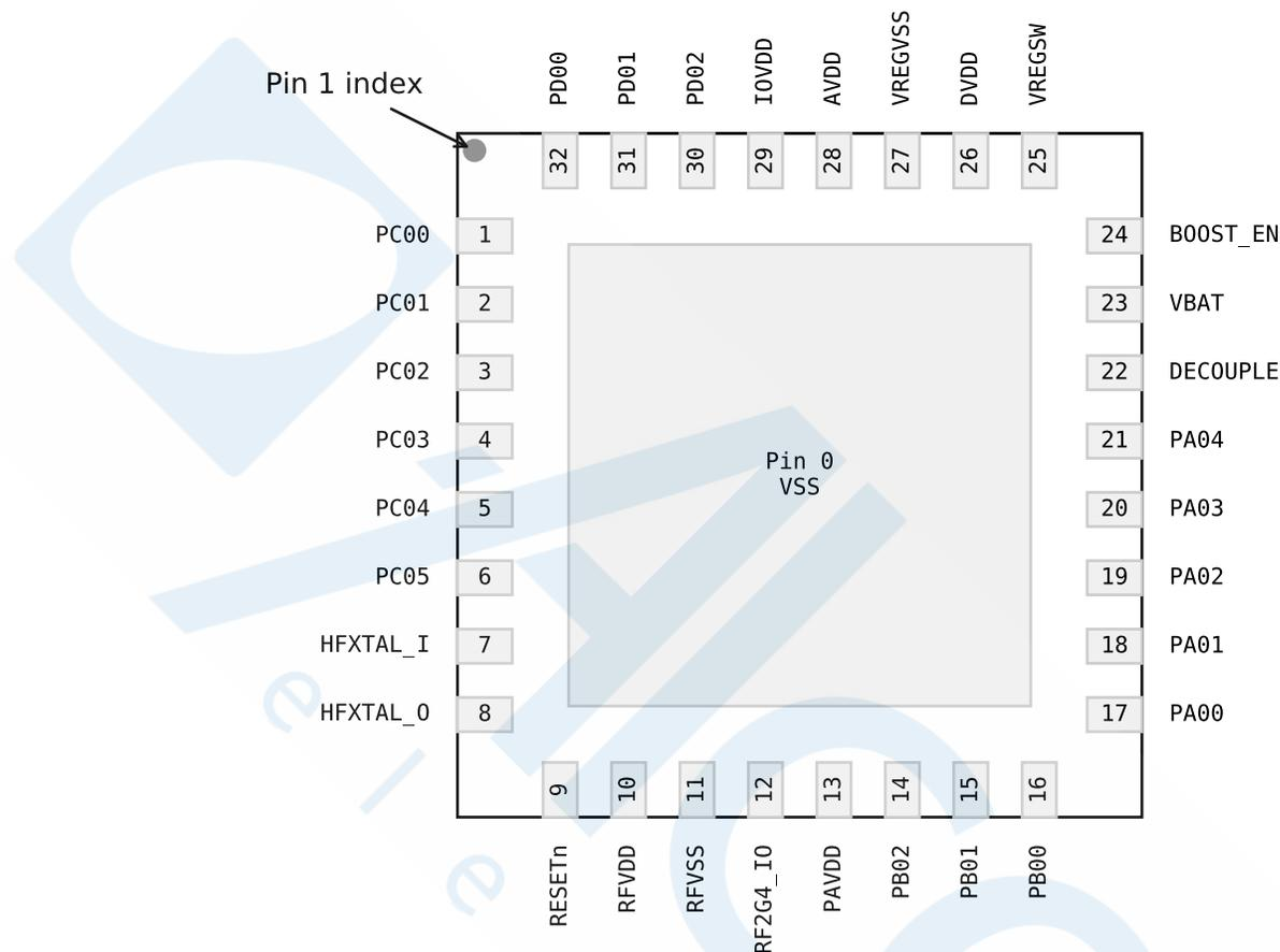
**Figure 6.4. QFN32 with Boost DC-DC Device Pinout**
