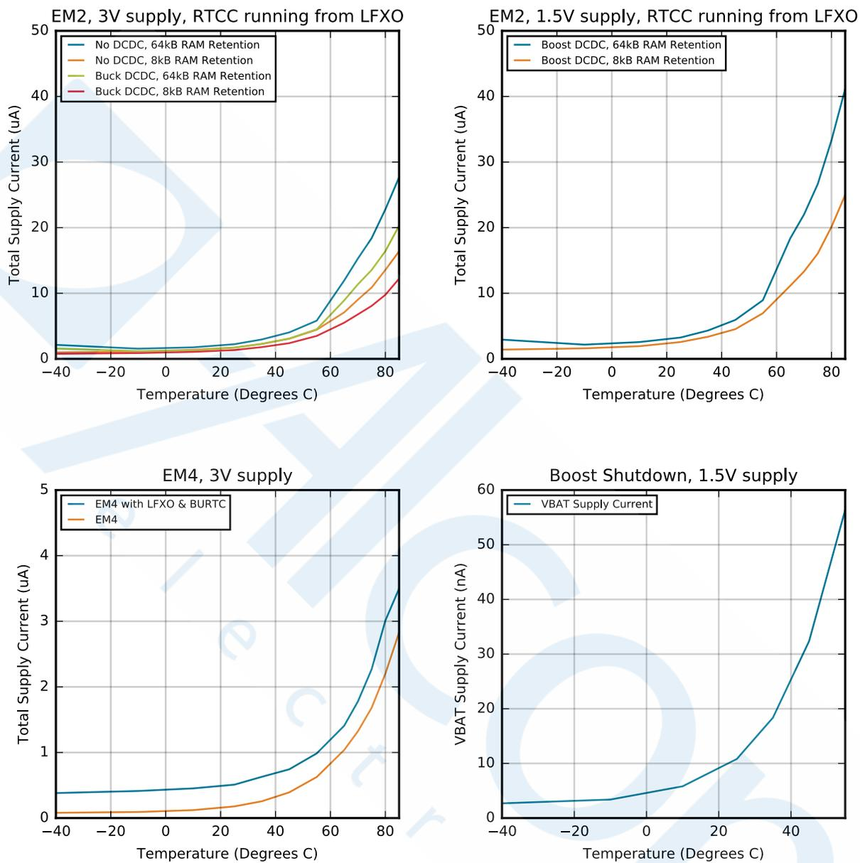
Figure 4.11. EM2, EM4, and Boost Shutdown Typical Supply Current vs. Temperature
