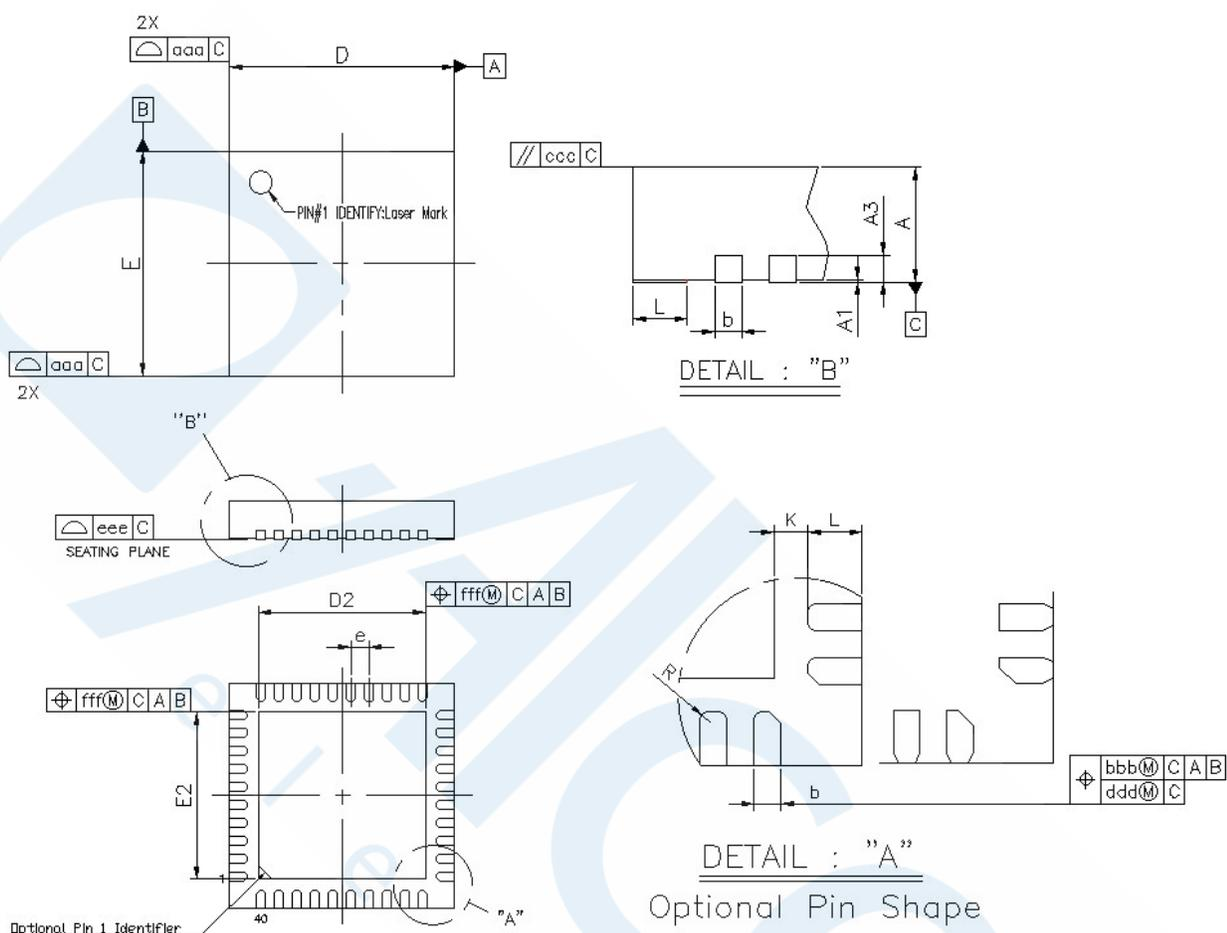
Figure 8.1. QFN40 Package Drawing
