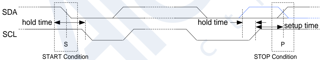
Figure 29. START and STOP (or repeated START, blue line) condition
