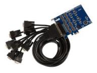
Sealevel PCI Express serial boards utilize 120-byte FIFOs for maximum reliability in data-intensive applications. Software developed for standard PCI boards will also work with Sealevel PCI Express boards, simplifying your transition to this next-generation PCI bus. Sealevel PCIe serial boards are configurable for RS-232, RS-422, and RS-485 electrical interfaces. These PCIe serial boards are fully compatible with X2, X4, X8, X16, and X32 PCI Express slots.
