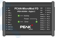
Figure 1: Top view PCAN-MicroMod FD Digital 1/2 with pin assignment
