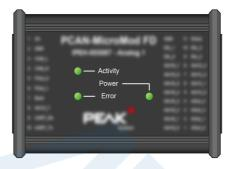
Figure 4: LEDs on the PCAN-MicroMod FD Digital 1/2
