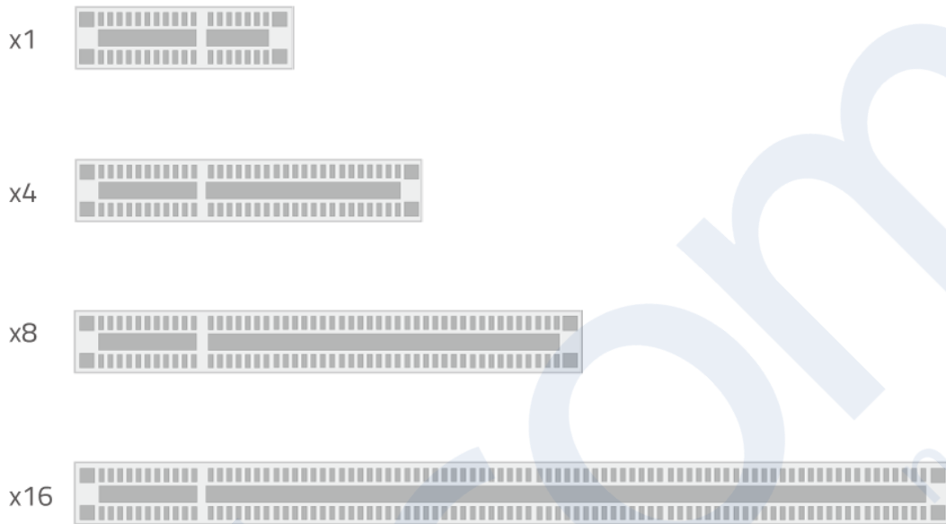
Different Types of PCIe Slots
