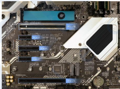
Different PCIe and PCI slots on a Motherboard
