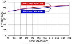
Efficiency vs. Input Voltage XL180-24 with Forced air cooling
