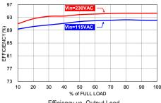
Efficiency vs. Output Load XL180-24 with Forced air cooling
