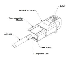
The MTCT300 uses a split-core current transformer to allow easy installation on existing wiring.
