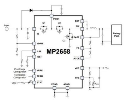
The MP2658 can be configured to different pre-charge to fast charge thresholds and different charge termination modes via the external pins. This allows the device to support super capacitor charging, as well as charging for different battery chemistries.
