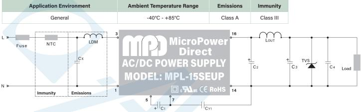
The diagram above illustrates a basic connection of the MPL-15SEUP series. The recommended components are given in the table below.
