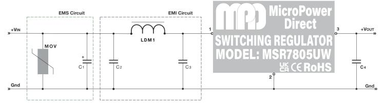
The diagram above illustrates a typical connection of the MSR7805UW(L) series for applications that require meeting EMC standards. An external MOV is recommended on the input to protect the unit in the event of a surge.
