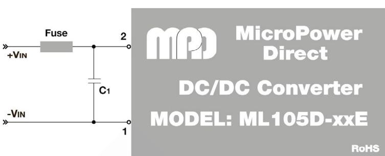
The diagram above illustrates a simple connection of the ML100xE series. For applications that do not require the circuit to meet EMi/EMC specifications, the capacitors C1, C3 and C4 will reduce input/output ripple and improve the converter stability over time and temperature. The recommended component values are given in the table at right.
