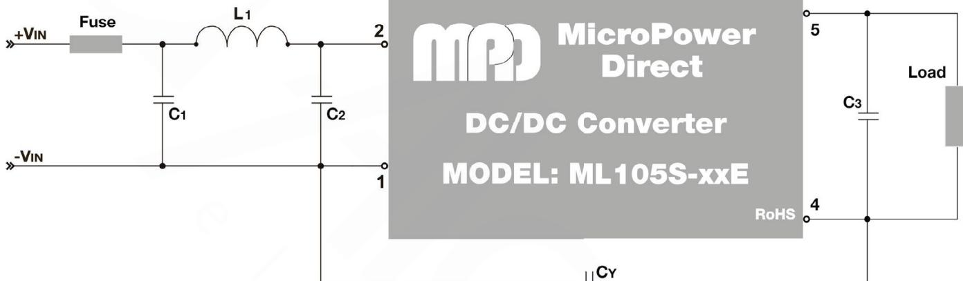
The diagram above illustrates a typical connection of the ML100xE series for an application that requires compliance to EMi/EMC standards EN 55032 and EN 61000-4 (as specified on page 1). Some notes on these components are:
