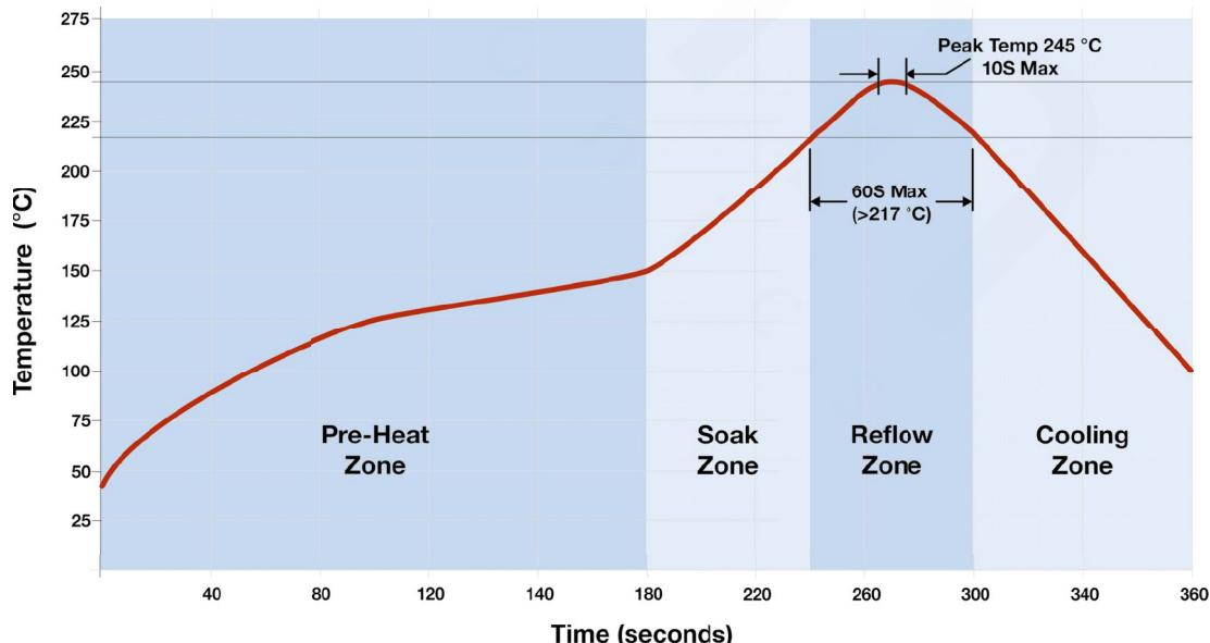
The ML100xE series is designed to meet the IPC/JEDEC standard J-STD-020D for reflow soldering. The recommended reflow settings are a peak temperature of 245 °C for a maximum period (TPK) of 10S and a time above liquidous (TL) of  $\leq$ 60 seconds at 217 °C, as illustrated above. For more information, please contact the factory.
