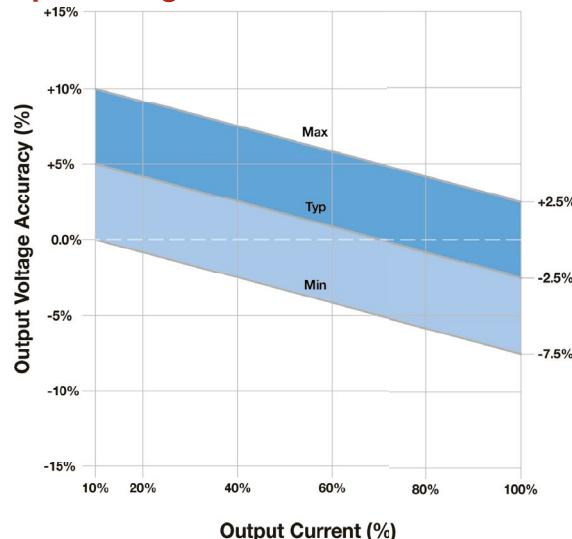
**Output Voltage Tolerance: 5 VIN, 3.3 VOUT**
