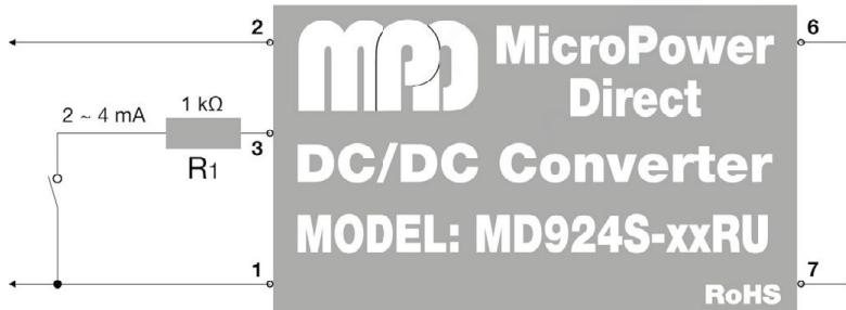
The MD900x-RU may be started or shutdown by the control pin (pin 3). This input is current controlled. The unit operates when this input is left open. When the input is "high" (current is flowing into the pin), the converter shuts down. The input current to this pin must be kept between 2 mA to 4 mA.
