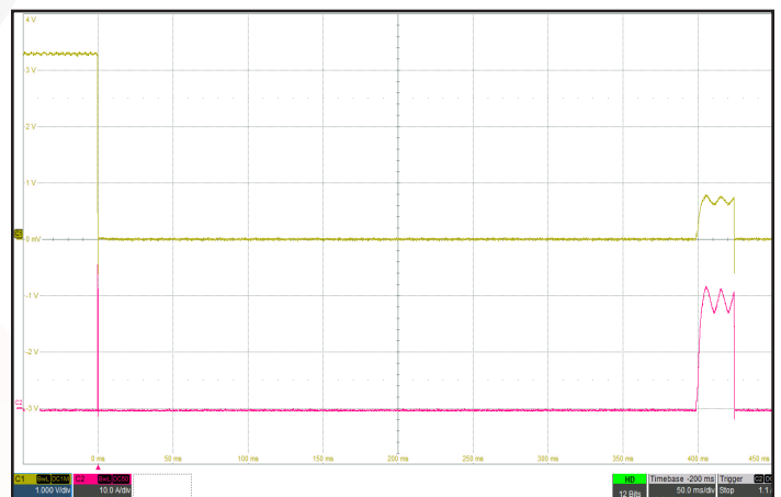
Figure 18: A short circuit across the output terminals. Ch 1: V_{out} (1 V/div). Ch 2: I_{out} (10 A/div).
