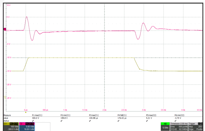
Figure 12: Output voltage response to step-change in input voltage (200 V - 300 V - 200 V) in 150 µs. Ch 2: Vout (5 V/div). Ch 1: Vin (100 V/div). Timescale: 500µs/div.
