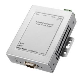
The JetPort 5601 is a RS-232/422/485 to Redundant Ethernet Serial Device Server. The serial interface is configurable in software and supports speed as fast as 921.6kbps. Dual Ethernet ports can support RTTD (Redundant to the Device) that can auto-recover in less than 200ms if the primary link breaks, as a result guaranteeing a non-stop connection. JetPort 5601 is also equipped with two types of power inputs, the terminal block and power jack.
