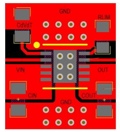
Figure 4. Recommended PCB Layout
