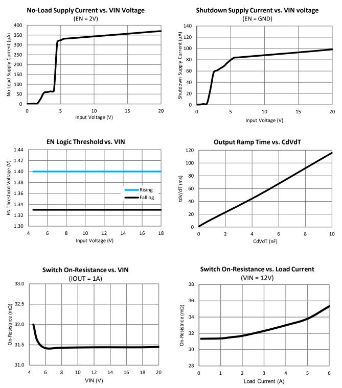
$V_{IN}$  = 12V, EN = 2V,  $R_{LIM}$  = 100k $\Omega$ , CdVdT = Open,  $C_{IN}$  = 1 $\mu$ F,  $C_{OUT}$  = 1 $\mu$ F, and  $T_A$  = 25°C, unless otherwise specified.
