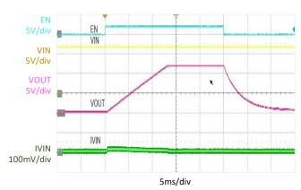
CLP followed by Thermal Shutdown and Restart (5.1A Current Limit, Riset =  $150k\Omega$ )
