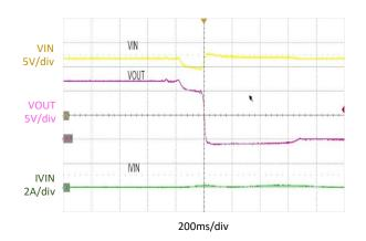
Enable Turn-on, Turn-off Response (No load, Cout =  $10\mu$ F, CdVdT = 1nF)
