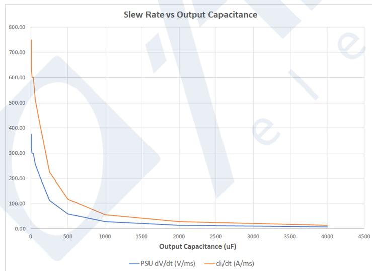
**Figure 5 - Slew Rate versus Output Capacitor**
