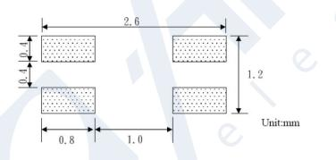
Available sizes: HDRC2012M HDRC1210 HDRC3216M HDRC3225M HDRC4520M HDRC4532M HDRC7060M
