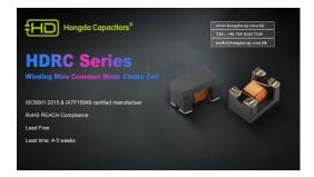
The HDRC2012 series Common Mode Choke Coil package size is 2.0x1.2x1.2mm, and the common mode impedance is  $30-1000\Omega$ . The main material of this product is a ferrite skeleton, and the enameled copper wire wound in parallel is a closed magnetic circuit chip structure, which has a good suppression effect on common mode noise, especially suitable for high-speed signal lines and high-current audio equipment.
