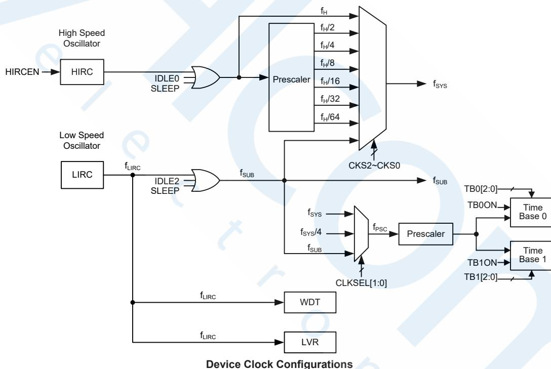
Note: When the system clock source  $f_{SYS}$  is switched to  $f_{SUB}$  from  $f_H$ , the high speed oscillator will stop to conserve the power or continue to oscillate to provide the cloak source,  $f_H \sim f_H/64$ , for peripheral circuit to use, which is determined by configuring the corresponding high speed oscillator enable control bit.
