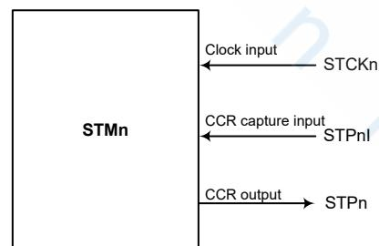
STM<sub>n</sub> Function Pin Block Diagram (n=0~1)
