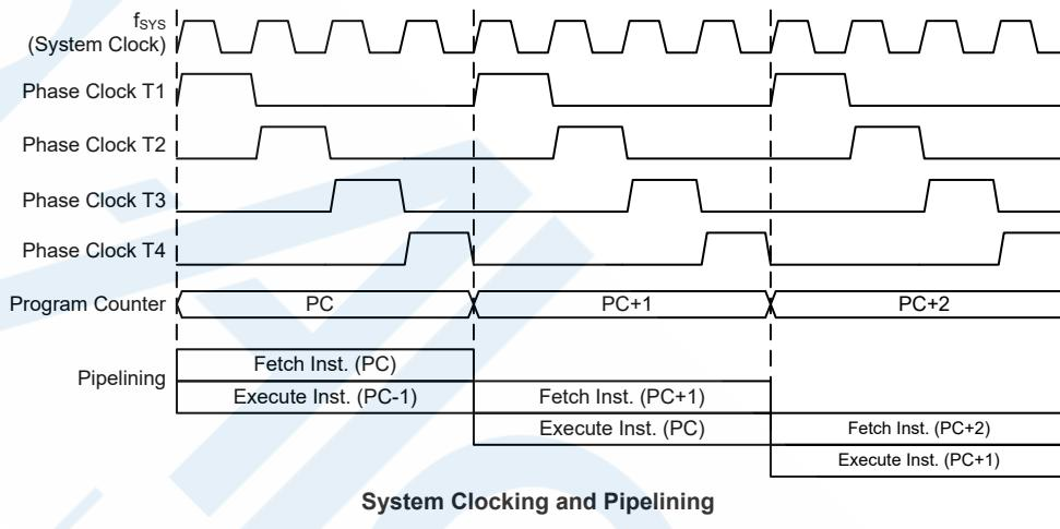
System Clocking and Pipelining
