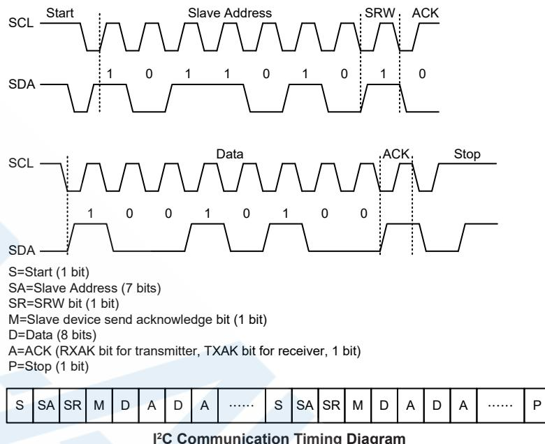
Note: When a slave address is matched, the device must be placed in either the transmit mode and then write data to the SIMD register, or in the receive mode where it must implement a dummy read from the SIMD register to release the SCL line.
