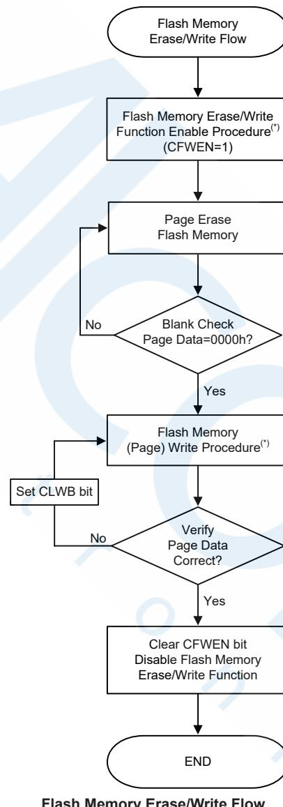
Note: The Flash Memory Erase/Write Function Enable procedure and Flash Memory Write procedure will be described in the following sections.
