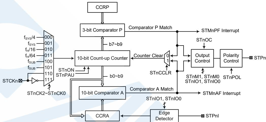
Note: The STM<sub>n</sub> external pins are pin-shared with other functions, so before using the STM<sub>n</sub> function, ensure that the relevant pin-shared function registers have been set properly to enable the STM<sub>n</sub> pin function. The STCK<sub>n</sub> and STPnI pin, if used, must also be set as an input by setting the corresponding bits in the port control register.
