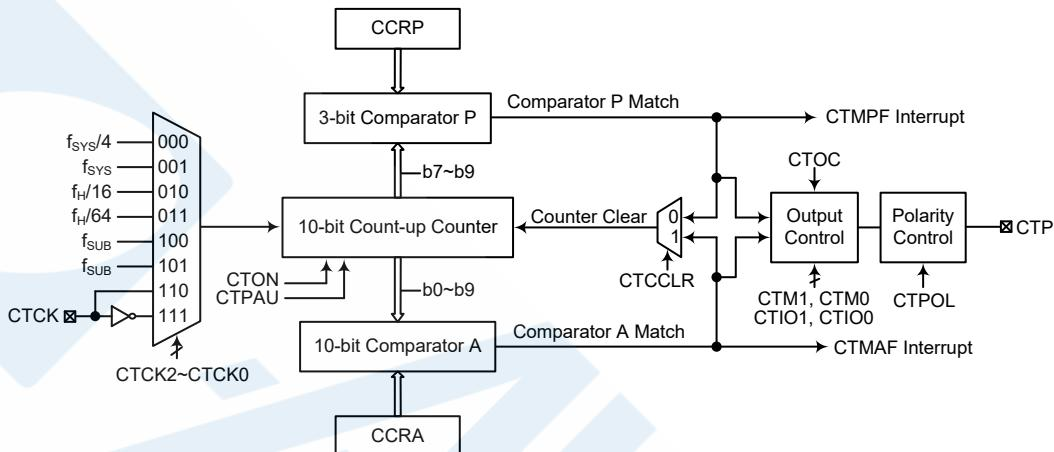
Note: The CTM external pins are pin-shared with other functions, so before using the CTM function, ensure that the relevant pin-shared function registers have been set properly to enable the CTM pin function. The CTCK pin, if used, must also be set as an input by setting the corresponding bit in the port control register.
