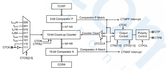
Note: As the CTM external pins are pin-shared with other functions, before using the CTM function, make sure the corresponding pin-shared function registers be set properly.
