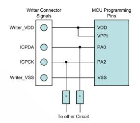
Note: \* may be resistor or capacitor. The resistance of \* must be greater than  $1k\Omega$  or the capacitance of \* must be less than 1nF.
