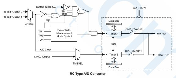
In the RC type A/D Converter mode, the timer A clock source is recommended to come from the system clock by configuring the TM[1:0] bits as 10. The timer B clock source comes from the external R to F oscillator or internal 128kHz LIRC2 oscillator selected by the TMBSEL bit in the ADCR register. The OVB\_OVAB bit in the ADCR register determines whether timer A or timer B overflows, then the RTMRF bit is set and timer interrupt occurs.
