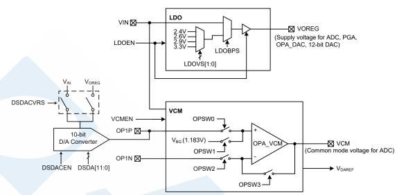
**Internal Power Supply Block Diagram**
