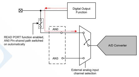
A/D Channel Input Path Internally Connection
