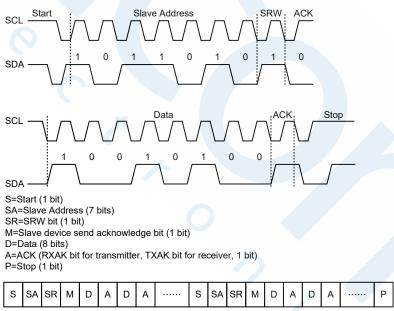
I<sup>2</sup>C Communication Timing Diagram
