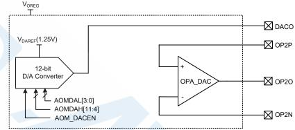
12-bit D/A converter and OPA Structure
