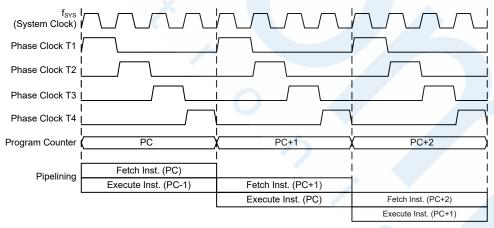
System Clocking and Pipelining
