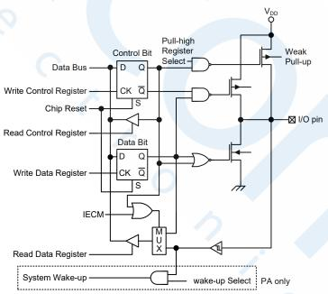
**Logic Function Input/Output Structure**
