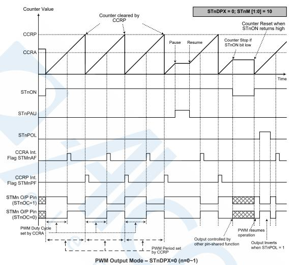
Note: 1. Here STnDPX=0 – Counter cleared by CCRP 2. A counter clear sets the PWM Period
