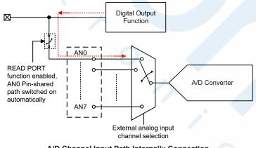
A/D Channel Input Path Internally Connection
