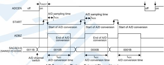
A/D Conversion Timing – External Channel Input
