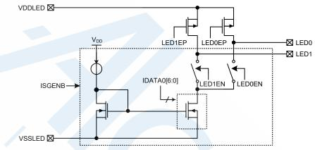
Sink Current Generator Block Diagram
