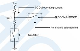
Software Controlled LCD Driver Structure
