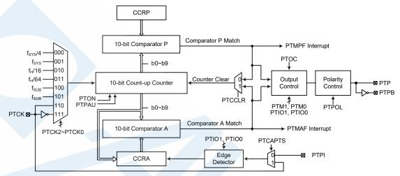
Note: The PTM external pins are pin-shared with other functions, so before using the PTM function the pin-shared function registers must be set properly to enable the PTM pin function.
