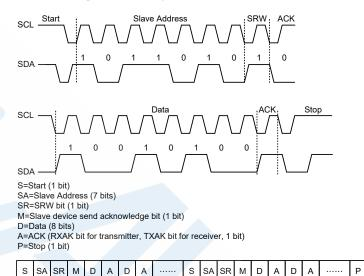
Note: When a slave address is matched, the device must be placed in either the transmit mode and then write data to the SIMD register, or in the receive mode where it must implement a dummy read from the SIMD register to release the SCL line.
