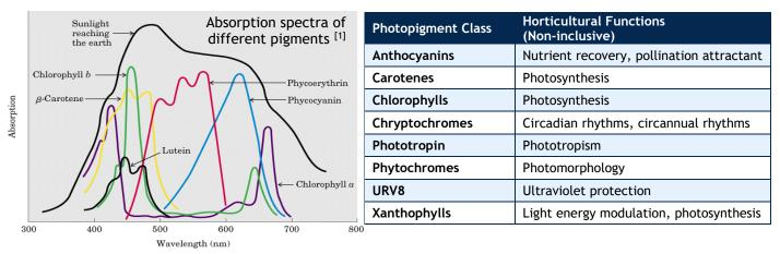
There is no single best solution for all horticultural applications. Different types of plants have different optimal light recipes. Luminus offers LED products with a wide range of light spectrums that can be combined to optimize growth phases.
