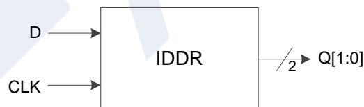
Figure 3-16 I/O Logic in DDR Input Mode
