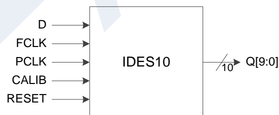
Figure 3-24 I/O Logic in IDES10 Mode
