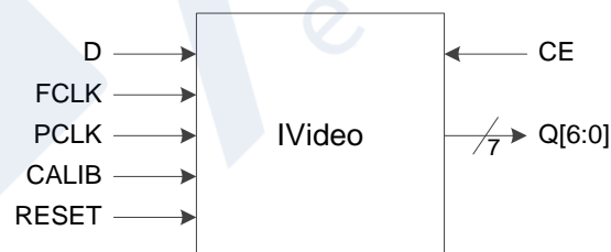
Figure 3-20 I/O Logic in IVideo Mode
