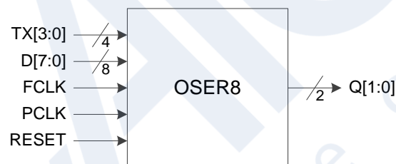
Figure 3-23 I/O Logic in OSER8 Mode
