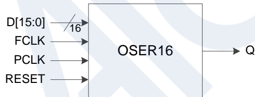
Figure 3-27 I/O Logic in OSER16 Mode
