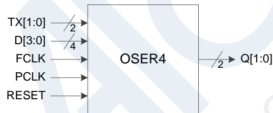
Figure 3-19 I/O Logic in OSER4 Mode
