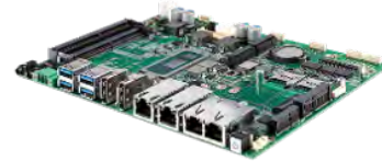
EXBC-1000 (5.25" SBC) Intel C246/H310 (CFL-R S/CFL-S) 10G USB 3.1 Gen 2, GigE LAN, RS-232/422/485, PCIe, SUMIT A, B
