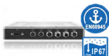
RES-3000 (M12) (Whiskey Lake-U) 2-port X-coded M12 LAN, M12 Power 2-port M12 COM, 2-port M12 USB
