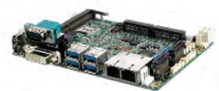
EMBC-1000 (3.5" SBC) Intel Core i7/i5/i3 SoC (Sky- lake-U) 5 COM, SUMIT A, B, 9V to 36V DC-in
