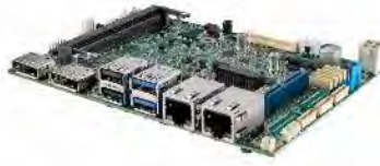
EMBC-5000 (3.5" SBC) Intel SoC (Tiger Lake) 10G USB 3.1 Gen 2, GigE LAN, 2.5G LAN, SUMIT A, B, 9V to 55V, Ignition Control
