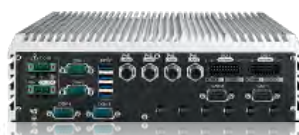
IVH-9200MXC (KBL-S/SKL-S) X-coded/A-coded M12 PoE+, 4 SSD Tray, 2-port CAN Bus
