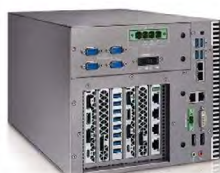
GPC-1000 (Dual GPU) (CFL-R S + Dual 2-Slot NV/AMD PEG) 9V - 55V, max 1500W for PEG, 4 PCIe
