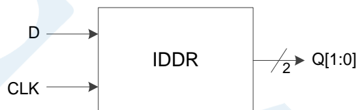
Figure 3-18 I/O Logic in DDR Input Mode
