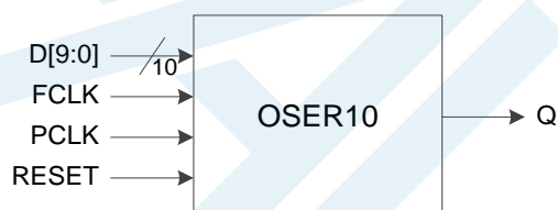
Figure 3-27 I/O Logic in OSER10 Mode
