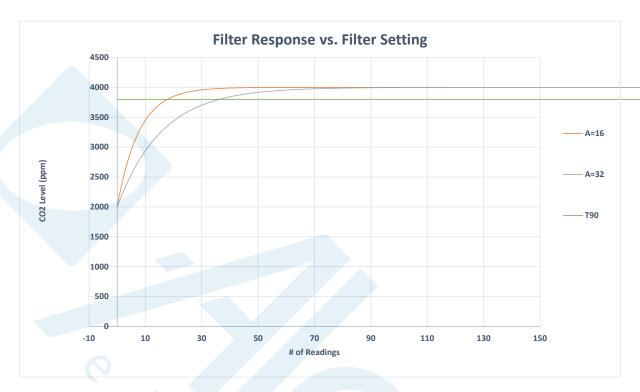
The graph above shows the effect of the filter on response times. Increasing the filter setting increases the measurement output response time.  $T_{90}$  is the time to 90% of reading. The CozIR®-LP3 takes 2 readings per second. The CozIR®-LP3 sensor will also output the raw unfiltered  $CO_2$  measurement data. This data can be post processed using alternative filter algorithms.
