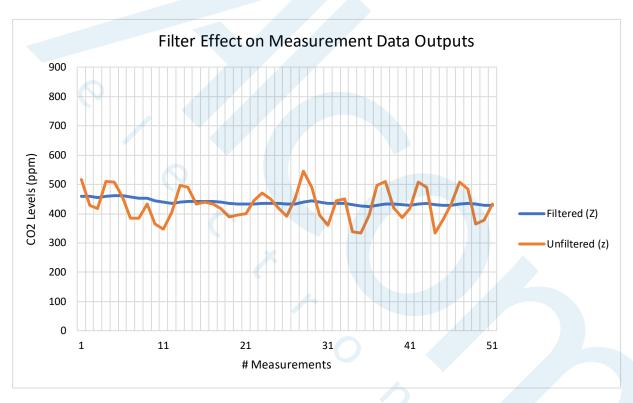
The graph above shows the effects of the filter on the CO<sub>2</sub> measurement data (Z). The unfiltered output (z) is shown in orange and the filtered output (Z) shown in blue.
