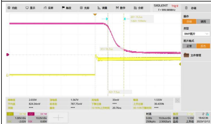
Figure 7-1 Turn-on Time Testing Waveforms
