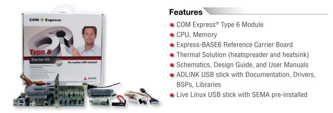
The starter kit plus consists of a COM Express<sup>®</sup> Type 6 core module with ATX size reference carrier board that offers one PCIe x16 Express slot with proprietary pinout for DDI Adapter card, one PCI Express graphics slot x16, One PCI Express x4 slot and three PCI Express x1 slots, Serial ATA, VGA, LVDS, USB 3.0/2.0, Gigabit LAN, and Super I/O. All necessary cables are included.
