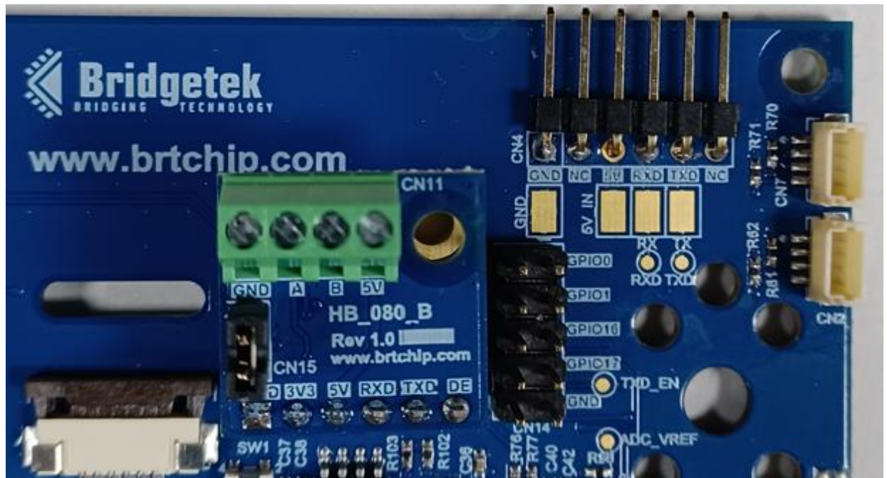
Figure 8 – IDM-RS485 Daughter Board Mounting Orientation
