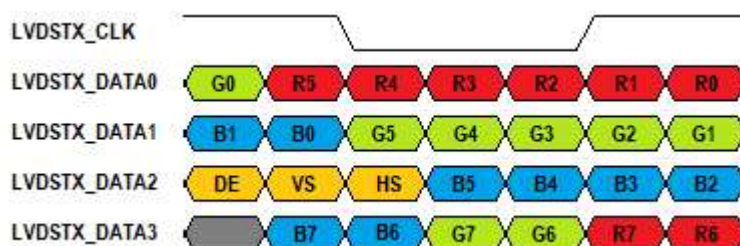
Figure 4 – VESA / Format 2 Mapping for 24-bit RGB
