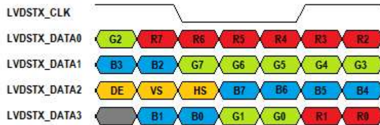
Figure 5 – JEIDA / Format 1 Mapping for 24-bit RGB
