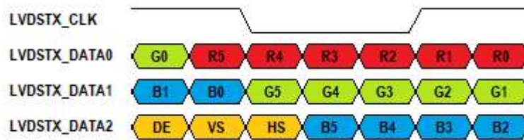
Figure 6 – JEIDA / Format 1 Mapping for 18-bit RGB
