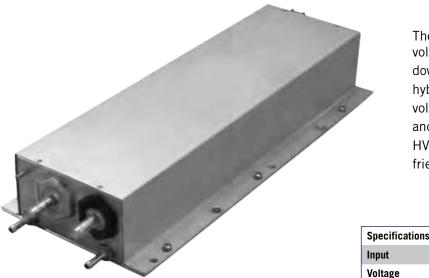
The 4000W LSM power module is a high voltage liquid cooled DC-DC converter which steps down 400V and provides 24V output, common in hybrid and electric vehicle applications. The output voltage is electrically isolated from the input voltage and suits the conventional 24V accessories and HVAC system requirements of industrial and ecofriendly vehicles.
