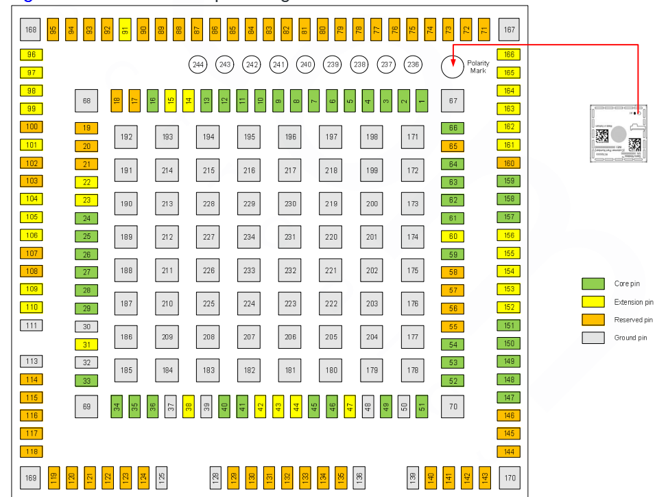
Figure 10-1: Pin Configuration (Top View, Through Module)
