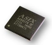
The AX88279 is a USB 3.2 Gen1 to 2.5G Ethernet controller with integrated 2.5G/1G/100M Base-T Ethernet PHY. AX88279 supports Precision Time Protocol (PTP), Microsoft Modern Standby, etc. advanced features, and supports Windows 11/10/8.x, Linux/Android/Chrome OS, Nintendo Switch in-box drivers, and macOS/Linux native CDC-NCM driver for driverless, Plug & Play.
