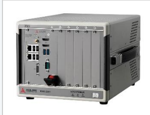
PXES-2301 6-Slot All Hybrid, PCIe Gen2, 8 GB/s
