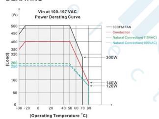
If input voltage is lower than 100VAC, please refer to the output derating V.S. input voltage curve for details
