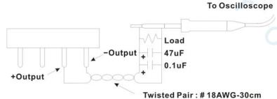
47uF and 0.1uF capacitor of proper polarity and voltage rating. The oscilloscope probe ground led should connect right to the ground ring of the probe and be as short as possible.
